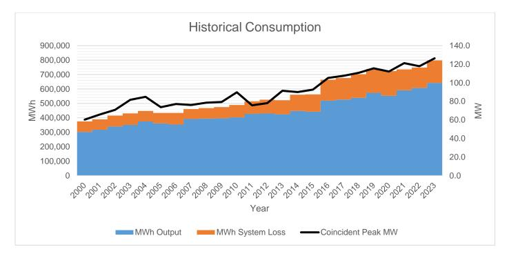
MWh output increased from 2000 to 2023 at an average rate of 3.61%, while MWh system loss from the previous year has increased at a rate of 10.10% due to both technical and non-technical losses. The EC still continues to plan and provide solutions to reduce its system loss by implementing system loss reduction programs and projects to rehabilitate and expand its distribution network.
