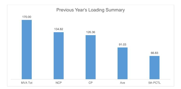
The Non-coincident Peak Demand is 134.82 MW, which is around 77.72% of the total substation capacity of 170 MVA at a power factor of 0.98. The load factor or the ratio between the Average Load of 91.03 MW and the Non-coincident Peak Demand is 67.52%. A safe estimate of the true minimum load is the fifth percentile load of 66.83 MW which is 49.57% of the Non-coincident Peak Demand.
