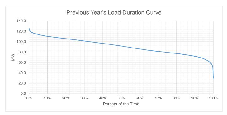
Based on the load duration curve, the demand most of the time is around 30 MW, and the maximum load is 126.36 MW from the last historical year.
