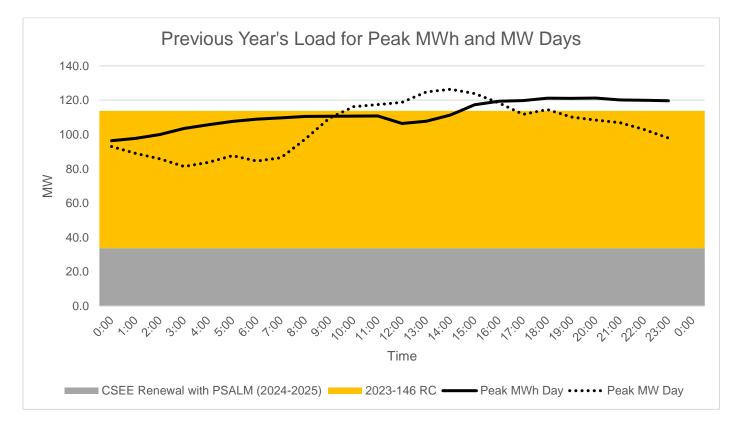
Peak MW occurred on May 12, 2023, at 2:00 p.m. due to high demand consumption during that time, and it was during the summer season. Peak daily MWh occurred on June 17, 2023, due to high energy consumption. As shown in the load curves, the available supply is lower than the peak demand, specifically during peak hours.
